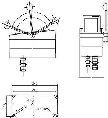
MH is handle type, having stepless speed regulation form with obvious hand touch, Ingress Protection is IP22.
