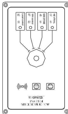
The content contacted via ATE is: transform for control position between wheelhouse control and local control, request and answer for SBE and FWE.
